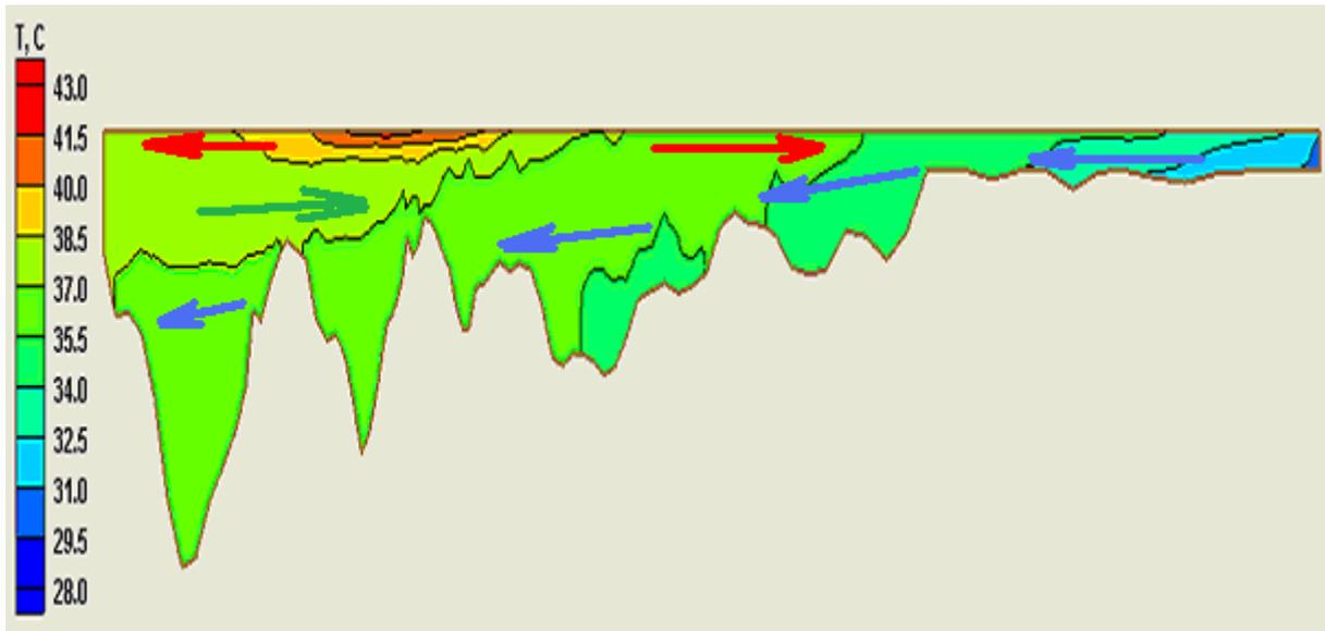
**Fig. 12. The circulation in the vertical section of the cooling pond in the direction from south to north. The red arrows show the flow of warm water, blue - return flow of cooled water. Green - the water flow at the intermediate level.**
