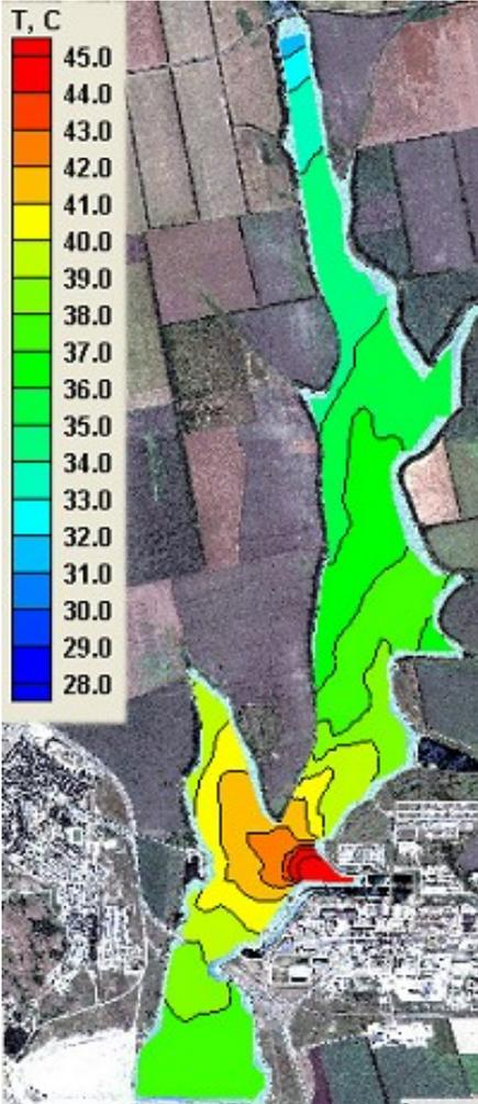
**Fig. 7. The distribution of surface temperature during work of 3 units of SU NPP with full capacity at the existing configuration of the cooling pond**
