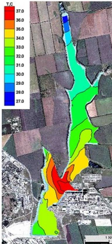
**Fig. 13. The distribution of surface temperature when working with 2 units of SU NPP (water heating is by 8°C) with the existing configuration of the cooling pond**
