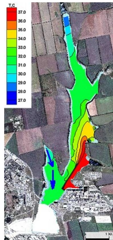
**Fig. 11. The distribution of surface temperature for the same configuration as in Fig. 9, but with training dike**
