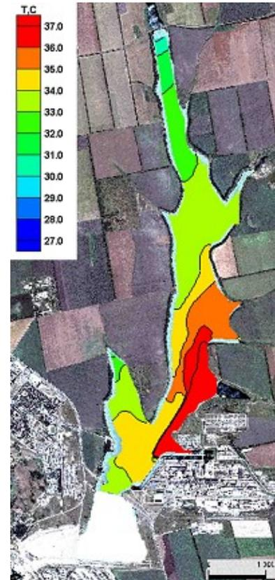
**Fig. 15. The distribution of surface temperature when working with 2 units of SU NPP units at full power (water heating is by 8°C) with the existing configuration of the cooling pond and construction of the dam for HSPS and training dike.**
