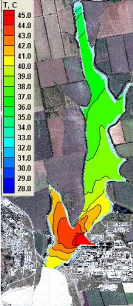
**Fig. 8. The distribution of surface temperature during the work of 3 units of SU NPP to full capacity after the construction of the dam for the needs of HPSPS**
