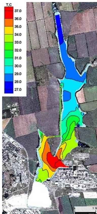
**Fig. 10. The distribution of surface temperature for the same configuration as in Fig. 9, but with a bypass channel**
