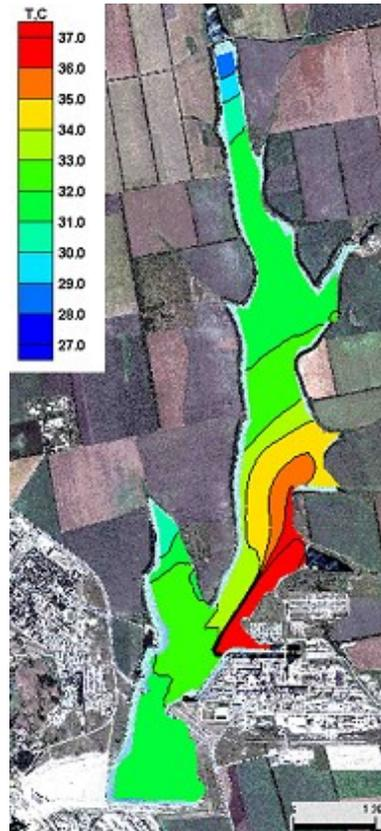
**Fig. 14. The distribution of surface temperature when working with 2 units of SU NPP units at full power (water heating is by 9°C) with the existing configuration of the cooling pond and construction of the training dike.**
