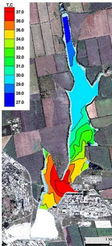
**Fig. 9. The distribution of surface temperature for the same configuration as in Fig. 8, but with the existing spray pond**
