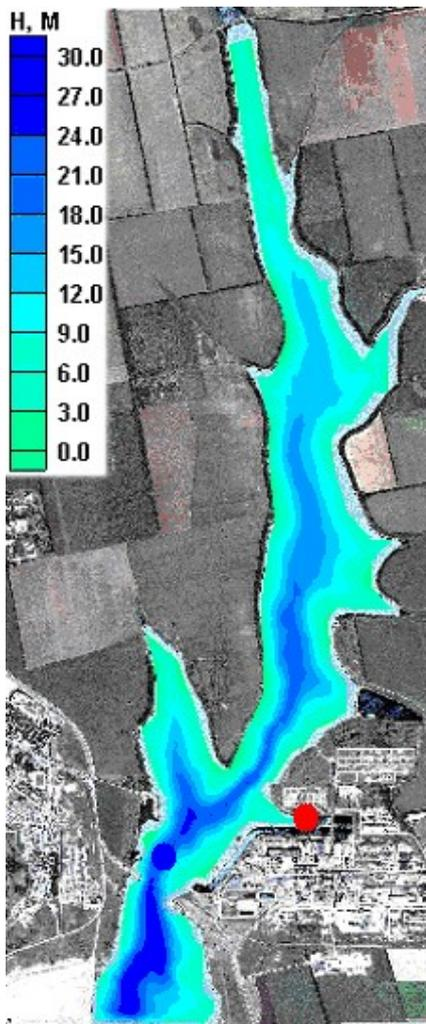
**Fig. 2. Topography of the cooling pond of SU NPP. Effluence of hot water is marked with a red circle, and blue is a deep water bottom intake.**
